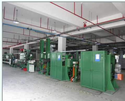
Extrusion for jacket
