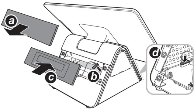
**Installing the Tango View Secondary LCD Display (Optional)**
