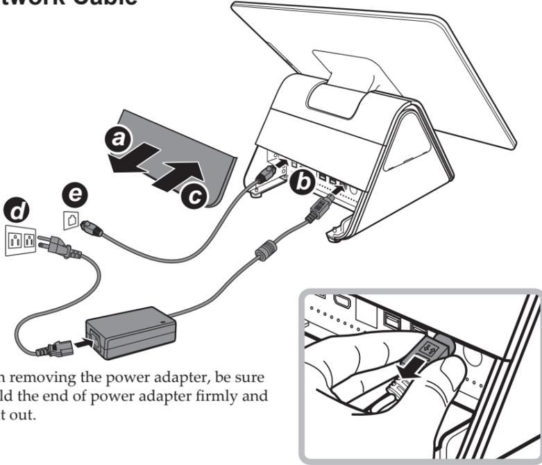
When removing the power adapter, be sure to hold the end of power adapter firmly and pull it out.
